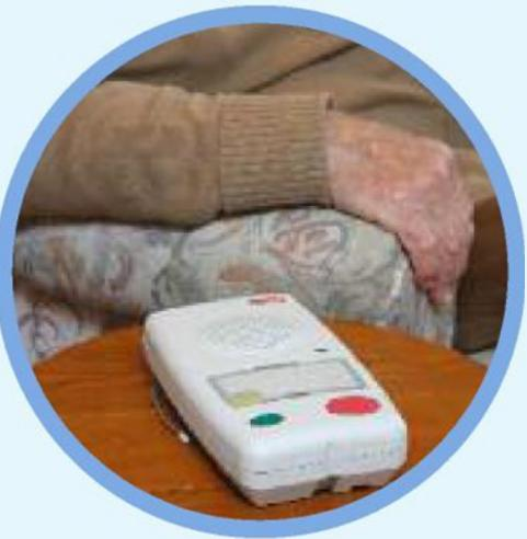
The system can give the unpaid carer peace of mind if they cannot be at home all the time because the sensor or button is connected to a monitoring centre which operates day and night. The monitoring centre staff will then contact you as the main carer to report as to what the problem is. A friend, or the emergency services, can also be consulted if you are not available.
