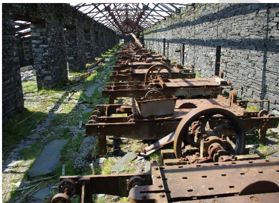
'Australia' Gallery Mill Saw Tables, Dinorwig Slate Quarry (Component Part 2) © Gwynedd Archaeological Trust
